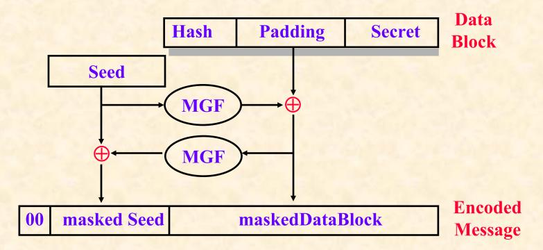
The encoded message is converted to an integer which is then encrypted using RSA.
